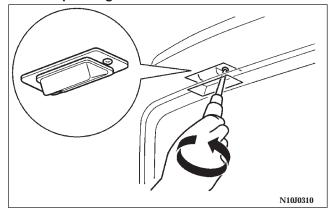
Remove the lens mounting screws, remove the socket assembly and the bulb together by turning it counterclockwise. And remove the bulb by pulling out.
